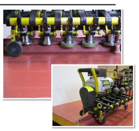
**NOTE:** When positioning the seamer onto the panel, ensure that the seamer is seated on the panel as shown *before* locking the handles into position. The 4th roller must be positioned on the hand-crimped area as shown below. **The seamer must be engaged in this manner. Failure to do so will result in panel damage.**
